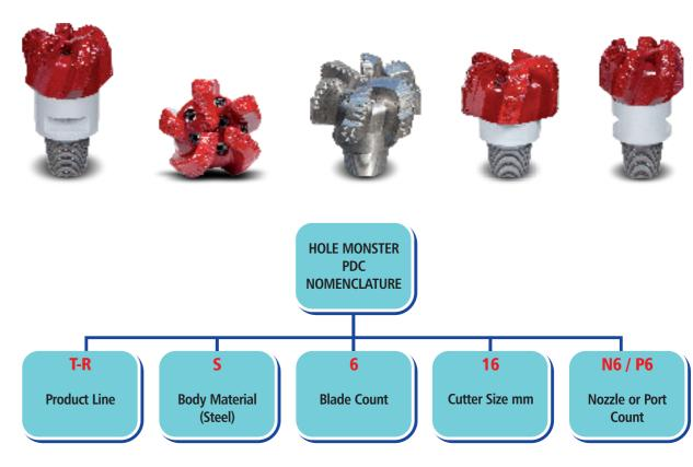
EXAMPLE: T-R S 616N6 (T-Rex type, Steel body, 6 Blades, 16mm cutters, 6 Nozzles)
